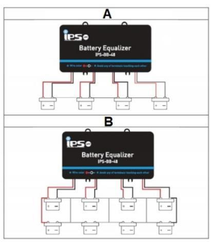
A - 4 batteries in a 48V (4\*12V) system
