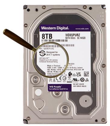
The Western Digital drives marked PURZ are designed to work in video surveillance systems. Its design allows for error-free recording of several Full HD streams in 24/7 mode.
