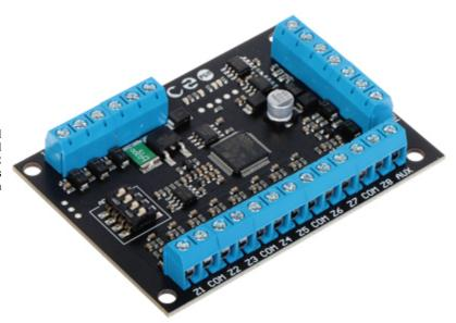
The device allows to expand the alarm control panel with additional 8 detection circuit inputs, 3 technical inputs for monitoring an additional power supply, 2 programmable outputs of OC type, 2 power outputs AUX and a tamper input for detecting the opening of an enclosure.
