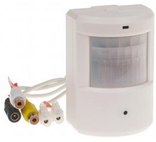
The color camera with Sony sensor with PIR detector built-in, hidden inside detector casing.
