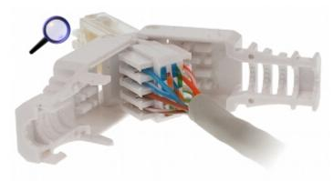
After placing the wires is enough to snap the connector:
