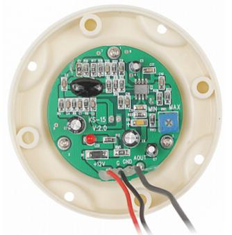
The device is equipped with a highly efficient, microprocessor dynamic compressor that adapts the level of amplification to the ambient noise level. Mounting side view:
