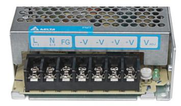
L - Live wire (230V) N - Neutral wire FG - Grounding -V - DC "-" output -V - DC "-" output +V - DC "+" output +V - DC "+" output ADJ - Output voltage adjustment Side view:
