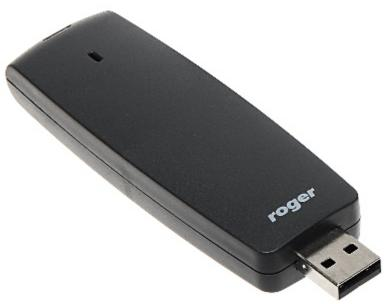
Proximity card reader connected to the computer's USB port for quick and convenient reading cards, keyfobs, etc. in RACS (min. ver 4.3), Roger MiniReader systems. For those who want to integrate RUD-2 with other software, the manufacturer provides a DLL library. A practical magnetic stand is included with the device.
