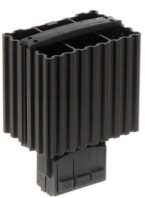
The HG-140-45W semiconductor heater operates based on a PTC thermistor. Heaters and fan heaters prevent condensation of water vapor and maintain the proper operating temperature of the devices. For optimum circulation of air it is advisable to install the convection heaters in the bottom part of the cabinet in a vertical position.
