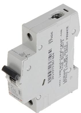
Thermal-magnetic circuit breaker with C-type curve and 10A rated current. The LE-419200 circuit breaker is compatible to DIN TS-35 rail mounting system. Circuit breakers with C-type breaking curve are designed to protection against short-circuits and overloads of the installation, where are used the devices with high inrush currents (motors, transformers).
