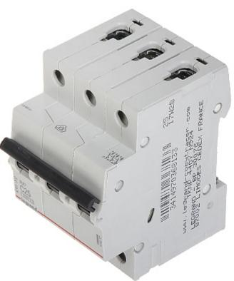
Thermal-magnetic circuit breaker with C-type curve and 25A rated current. The LE-419237 circuit breaker is compatible to DIN TS-35 rail mounting system.
