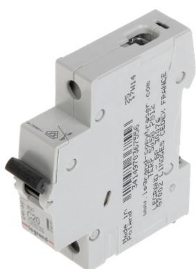
Thermal-magnetic circuit breaker with C-type curve and 20A rated current. The LE-419203 circuit breaker is compatible to DIN TS-35 rail mounting system. Circuit breakers with C-type breaking curve are designed to protection against short-circuits and overloads of the installation, where are used the devices with high inrush currents (motors, transformers).
