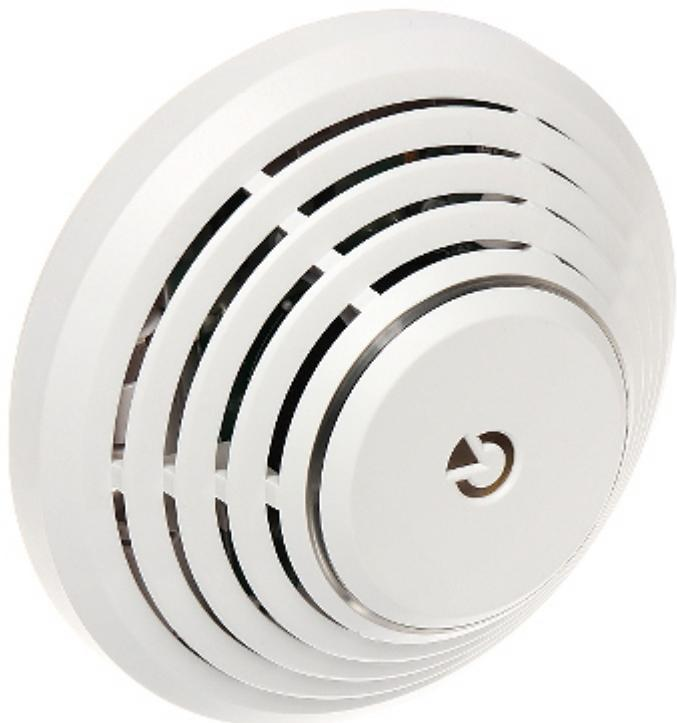
Smoke and heat detector allows to early detection of a developing fire. Alarm is triggered after detection of smoke and/or after the temperature rises above the critical value. The detector is powered from the alarm control panel bus, and if this power supply is lost, it is supported from the installed batteries (3x 1.5 V AA) and operates as an autonomous unit. The device is addressable, and occupies one address in alarm system.
