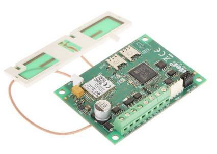
GPRS Communications Module for INTEGRA, INTEGRA Plus alarm control panels. The device allows to reporting to the monitoring station, remote programming and service, notifying the user and controlling the system by SMS, CLIP or INTEGRA CONTROL application running on iOS / Android systems.
