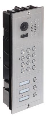
Video Doorphone is mounted in a flush-mounted housing. Surface mounting is possible with the D600B3 cover. Built-in code lock allows to control the opening state of two independent entrances with separate codes (eg wicket + automatic gate).
