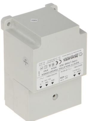
Single phase safety isolating transformer with short-circuit and thermal protection, is designed and made according to EN61558-2-6 norm. Transformer windings are isolated and sealed with polyurethane inside self-extinguishing housing.
