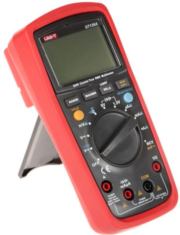
UT-139A is a universal digital meter used to measure: voltage, current, resistance. The meter has the function of automatic change of measuring ranges, as well as a relative measurement mode (when measuring voltage, current and resistance). The device also has a built-in battery tester.
