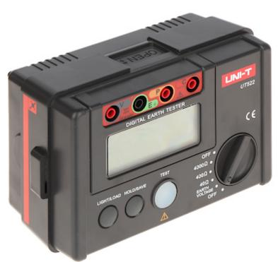
The UT-522 meter allows to measure: grounding resistance of power installations, grounding resistance of devices, resistance of lightning protection systems, etc. The design of the device allows for a complete, accurate measurement of the grounding resistance using 3 leads and a simple, approximate measurement using 2 leads.
