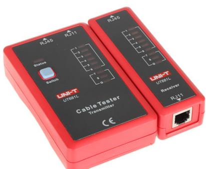
The UT-681L tester is designed to test the correctness of the cable terminating, wires sequence in RJ-45 and RJ-11 plug. The test can be made with two speeds. To test the cable the Main Tester must be connected to the one plug of the cable and the Remote to the other one. The device case is made from a solid plastic, which guarantees the reliability and long-term working during the installations.
