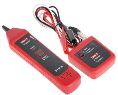
The UT-682D is a wire pair detector consisting of a transmitter and a receiver. The device allows you to perform measurements on telephone lines, twisted-pair cables and electric cables. The detector is designed to identify and search wires without disturbing their insulation. For telephone lines, it can additionally indicate the line status and facilitate troubleshooting of installation and maintenance.
