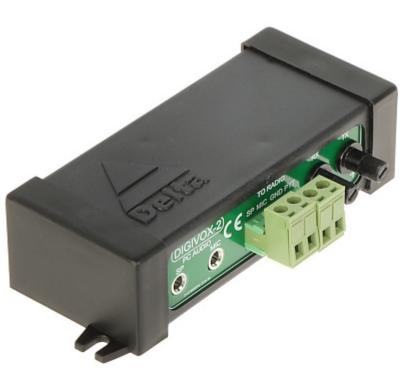
The DIGIVOX-2 is a passive, no power supply system that interfaces the computer with the radio. The device is designed for digital modes that use the sound card as a modem.
