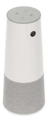
The A30T conference camera is a combination of a camera, microphones array and a loudspeaker into one device. The A30T camera with a resolution of 2.1 Mpx and wide view angle is ideal for conducting video conferences in small-to-medium-sized teams. The built-in 4-element omni-directional microphones array, customized, human-voice-optimized wide-band speaker, enable full-duplex two-way communication within 5 meters distance with the real feeling of stable sound.
