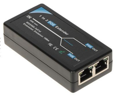
The PFT1320 device allows for connection of 2 cameras with PoE power supply using a single Ethernet line. The cascading connection of 2 extenders allows to connect up to 3 cameras in this way. The device is powered from the PoE switch or other device compliant with this standard. Thanks to this, neither the extender nor the camera connected to it require any additional power supply.
