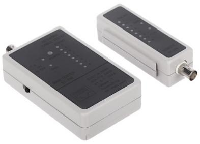
The ST-248 allows to check the proper install and the order of wires of the RJ-45 plug and can also tests if there is a signal between two ends of the coaxial cable with BNC plugs. The test can be made with two speeds. To test the cable the Main Tester must be connected to the one plug of the cable and the Remote to the other one. The device case is made from a solid plastic, which guarantees the reliability and long-term working during the installations.
