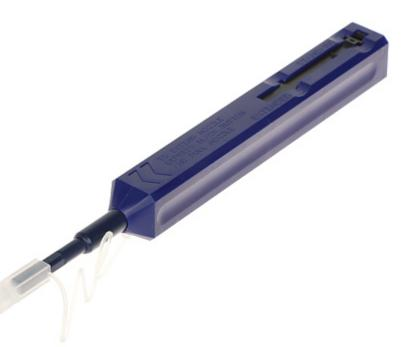
The WUN-XK125 tool is used to clean the end face of the ferrule in fiber optic connectors. A special fabric removes any contaminants, and its antistatic properties prevent dust from settling again. The product is suitable both for cleaning connectors in adapters mounted individually and mounted in patch panels.
