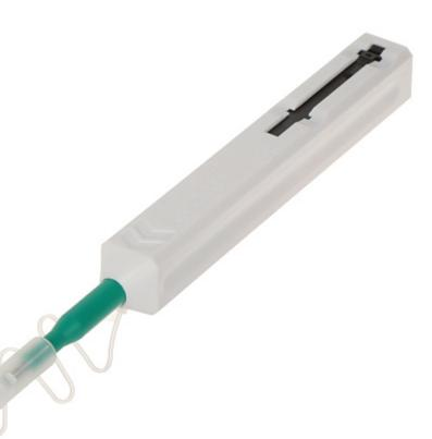
The WUN-XK25 tool is used to clean the end face of the ferrule in fiber optic connectors. A special fabric removes any contaminants, and its antistatic properties prevent dust from settling again. The product is suitable both for cleaning connectors in adapters mounted individually and mounted in patch panels.
