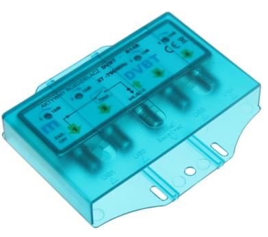
Active splitter with amplification adjustment. If antenna is without an amplifier, the device detects it automatically and does not pass the voltage to it. The device is perfect to installations, where length of the antenna cable from the splitter to the TV set is from several to several dozen meters (maximum 50m). Protection enclosure included in the kit enables outdoor installation, directly to the antenna mast.
