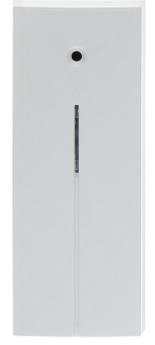
Sensor signals an alarm on registering a low-frequency tone (impact sound), followed by a high-frequency tone (sound of broken glass). The sensor starts to analyze a high-frequency channel after receiving the low-frequency sound wave, caused by the impact.
