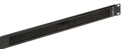
Width: 19 " Height: 1 U Material: Steel - powder painted Color: Black (RAL 9005) Application: RACK 19" + 389 x 30 mm (opening for cables entry) · Cable entry with brushes ensuring protection against dust Main features: • 4-point fixing to the front RACK rails • 4 pcs. of M6 screws with cage nuts included Corrosion resistance Weight: 0.225 kg Dimensions: 483 x 44 x 15 mm Guarantee: 2 years
