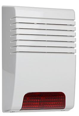
Outdoor siren with optical and acoustical signaling intended for use in intruder alarm systems. Optical signaling source are LEDs, and acoustical signaling is generating by piezo transducer.
