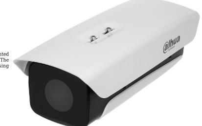
Half-open housings allow to easy access to inside mounted elements in contrast to sliding housings. Attention: The camera ground shouldn't be connected to the housing ground.
