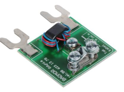
The SA/III-V-DIPOL antenna impedance transformer matches the antenna impedance to the impedance of coaxial cable.
