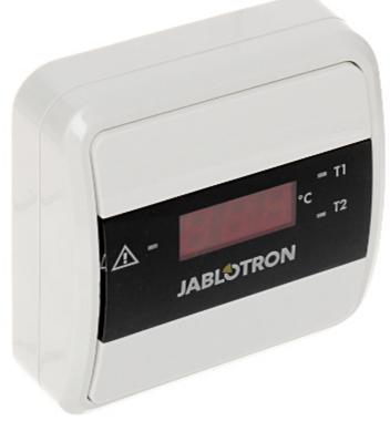
The TM-201A multi-function thermometer enables temperature measurement with using up to 2 sensors CP-201T-NW (available separately). The device can work as: thermometer indicating exceeding the preset temperature, monostable thermostat, bistable thermostat, differential thermostat.
