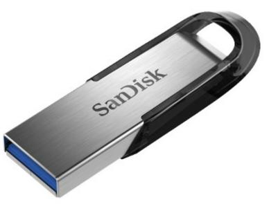
The SanDisk Ultra Flair USB flash drives are modern, compact and very efficient devices. Connectivity via USB 3.0 port enables up to 150 MB/s data read speed.
