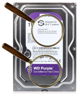
The Western Digital drives marked PURZ are designed to work in video surveillance systems. Its design allows for error-free recording of several Full HD streams in 24/7 mode.
