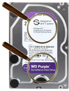
The Western Digital drives marked PURZ are designed to work in video surveillance systems. Its design allows for error-free recording of several Full HD streams in 24/7 mode.
