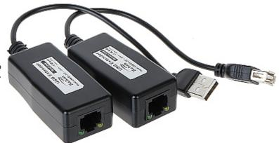
USB mouse extension over UTP Cat. 5/5e/6. Allows to control the DVR using USB mouse from remote location. Max. distance range is 100 m (USB 1.1).
