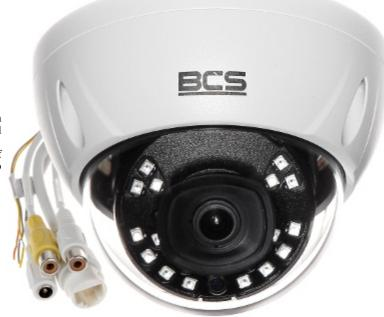
IP camera with efficient H.264 / H.265 image compression algorithm for clear and smooth video streaming at maximal resolution of 2688 x 1520 (4.0 MPx). PoE powering possibility, compatible with the 802.3af
