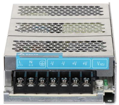
L - Live wire (230V) N - Neutral wire GND - Grounding -V - DC "-" output -V - DC "-" output +V - DC "+" output +V - DC "+" output ADJ - Output voltage adjustment Rear view:
