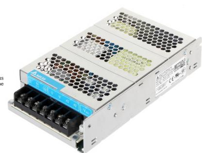
Power adapter with two pairs of output terminals. Attention! If the power adaptor is using for continuous work (24H) the rated current of the adaptor should be less than 80% of the maximal current.
