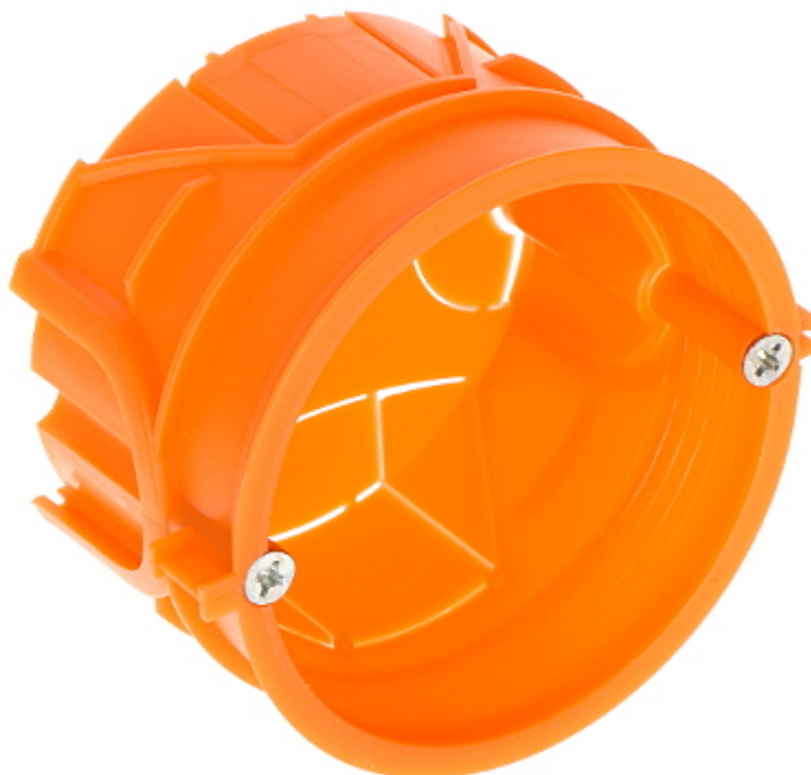
Flush mounting box. The box can be used as a single or combined in standard frame sets with spacing 71 mm.
