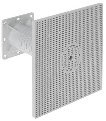
Mounting desk with electrical installation box for installing electrical devices (eg outdoor lights, motion sensors, etc.) on thermally insulated buildings facades with a thickness from 50 to 200 mm. The robust construction. Elimination of thermal bridging.
