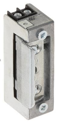
The electric strike of R4-24.13 type is designed for door and gates made from metal profiles, to work together with ratchet-latch or ratchet type door lock. It operates reversibly - it is open when power is off.
