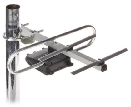
The 3/21-69 directional antenna is designed to receive DVB-T digital terrestrial television. For use at small distances from the transmitter. Some antenna parts are made from aluminum, steel construction elements are galvanized.
