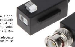
The PFM800B-4K is designed to video signal transmission via twisted-pair cable. The device adapts the impedance of coaxial cable  $75\Omega$  to the impedance of symmetrical line, ensuring transmission of video signal up to 400m (twisted-pair cable category 5) and eliminates asymmetric interferences.
