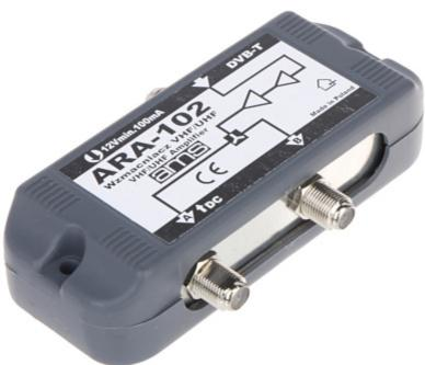
The ARA-102 is used to TV signal distribution in home antennas installations. Two-stage, low noise, distribution amplifier, allows to connect 2 TV sets to the antenna installation or cable network.
