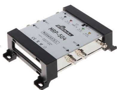
$\boldsymbol{Attention!}$  For unloaded outputs, use 75  $\boldsymbol{\Omega}$  terminating resistors.
