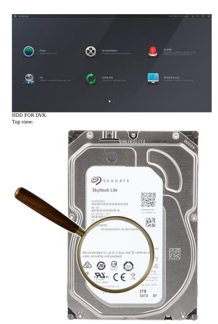
The Seagate drives marked SkyHawk are designed to work in video surveillance systems. Its design allows for error-free recording of several Full HD streams in 24/7 mode. Connectors:
