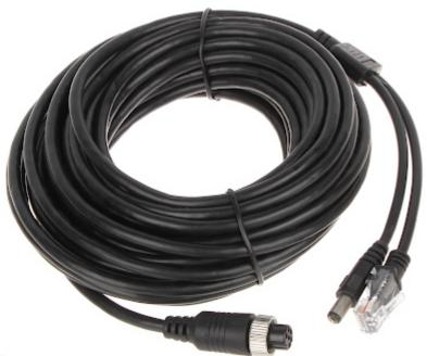
The connecting cable is terminated on one side with a M12 6-pin socket, and on the other with a RJ-45 plug and a 2.1/5.5 mm power plug.
