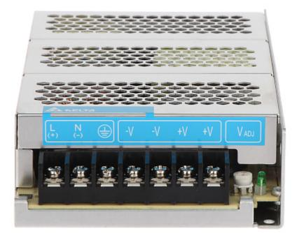
L - Live wire (230V) N - Neutral wire GND - Grounding -V - DC "-" output -V - DC "-" output +V - DC "+" output +V - DC "+" output ADJ - Output voltage adjustment
