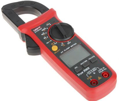
The UT-202A+ is a universal digital meter equipped with clamps enabling the measurement of high currents. The device measures: voltage, current, frequency, resistance and capacity. In addition, the meter has an electric field detection function (NCV).
